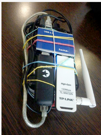
A portable wi-fi access point consisting of a Raspberry Pi mini-computer system, a UTMS aerial, a wi-fi aerial, a battery pack with a life of around two days, a USB port and a number of elastic bands
